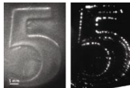
IMPRINT of the number "5" glows (right) thanks to an electronic sensor with human-touch sensitivity.
