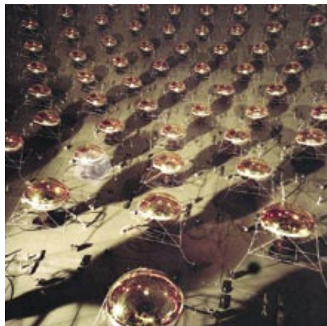
MULTIPLIER TUBES inside the MiniBooNE tank can detect the light produced from neutrino interactions.
